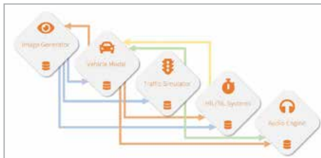
Fig. 1 - Each gray square represents a different software participant: the connections and data generated and used by the software rapidly becomes unmanageable
