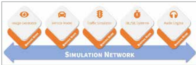
Fig. 2 - The Simulation Framework uses a common communication infrastructure or "Simulation Network" where each software connects through a Binding Node
