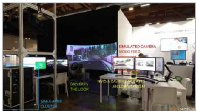
Fig. 7 - Demo of the AnteMotion framework at the Research Agora at the 2019 CAE Conference. An Image Generator in the simulator cluster generates a video feed for the nVidia Xavier System that is simulating an LDWS system. The driver in the loop can feel the torque on the steering wheel generated by the mockup of a real ADAS system
