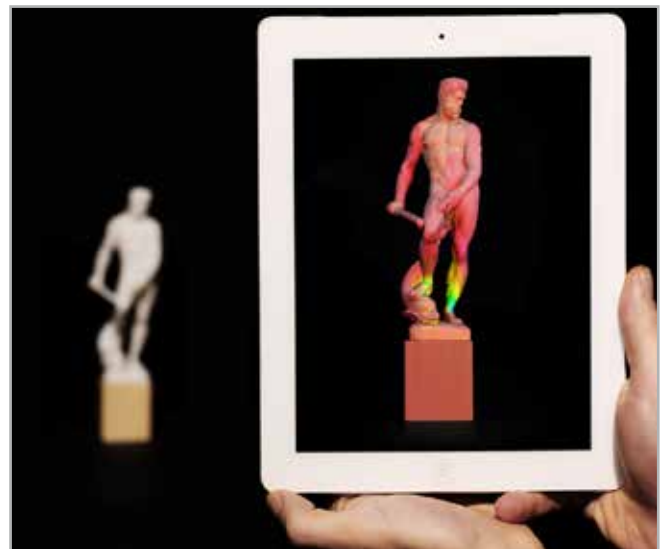
Fig.3 - Augmented reality: projection of seismic analysis on 3D print
