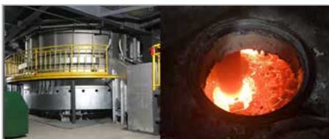
Fig. 1 - Left - Electric melter. Right - Detail of the fusion of basalt and dolomite rocks.
