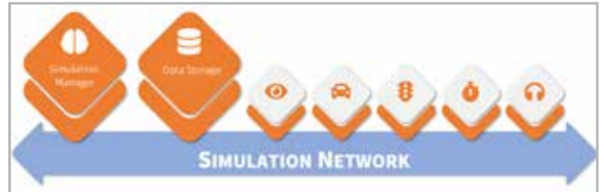
Fig. 5 - The simulation framework allows the introduction of additional management nodes, such as the Simulation Manager and Asset Database
